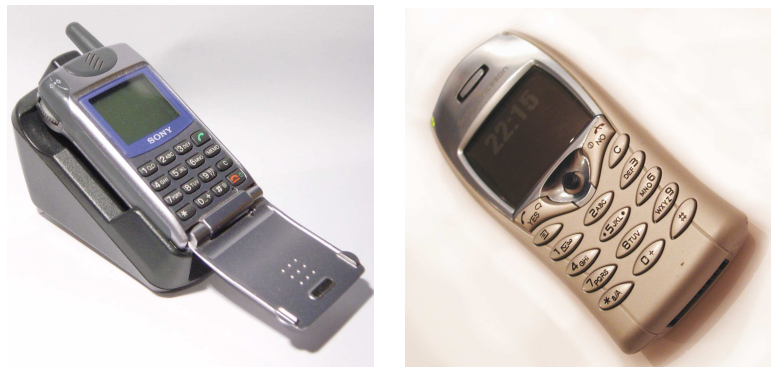
Figure 3.7: Sony Ericsson CMD Z5 with jog wheel and Sony Ericsson T68i with joystick.
