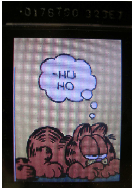
Figure 5.4: A comic strip shown on the display. The LCD's origin is in the upper right corner which caused the images to be mirrored on the y-axis in the first versions.
